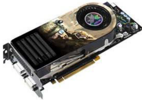
Asus GeForce EN8800GTX/HTDP/768M, 768 MB, dual DVI, TV-out
